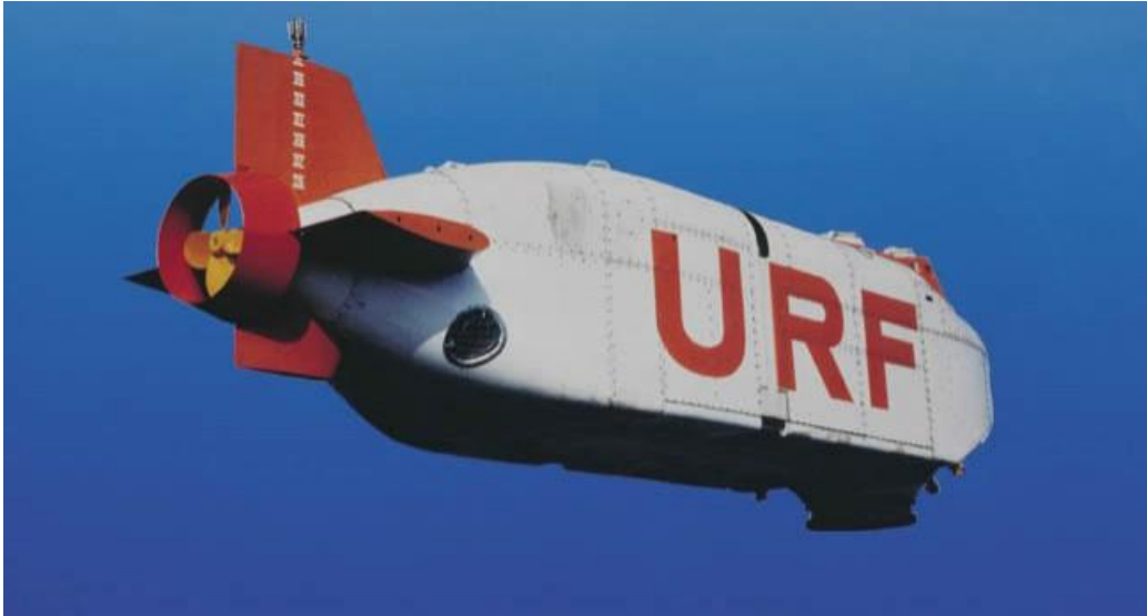
Figure 1.2 KAB's Submarine Rescue Vehicle (source: [3]).
